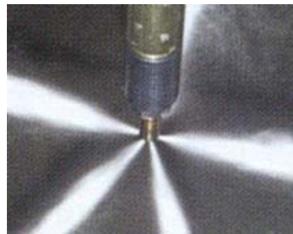
Clean injectors offer a uniform spray pattern
